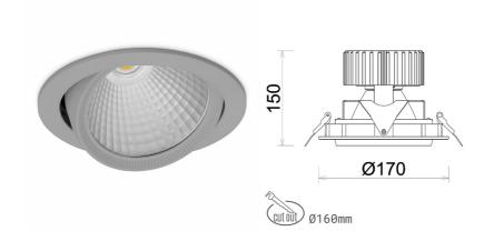
COB Light colour 3000 [K] | CRI Led chip flux 2994 [lm] Luminous flux 2395 [lm] System power 21 [W] Luminaire Efficiency 114 [lm/W] Beam angle 45° Controller ON/OFF MacAdam 3 SDCM
