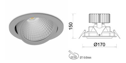
COB Light colour 3000 [K] | CRI Led chip flux 2994 [lm] Luminous flux 2395 [lm] System power 21 [W] Luminaire Efficiency 114 [lm/W] Beam angle 30° Controller ON/OFF MacAdam 3 SDCM
