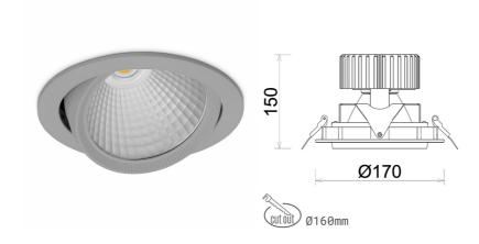
COB Light colour 3000 [K] | CRI Led chip flux 3811 [lm] Luminous flux 3048 [lm] System power 27 [W] Luminaire Efficiency 113 [lm/W] Beam angle 15° Controller ON/OFF MacAdam 3 SDCM
