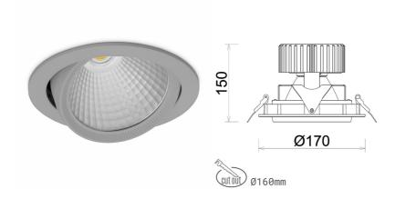
COB Light colour 2700 [K] | CRI Led chip flux 3772 [lm] Luminous flux 3017 [lm] System power 27 [W] Luminaire Efficiency 112 [lm/W] Beam angle 45° Controller ON/OFF MacAdam 3 SDCM
