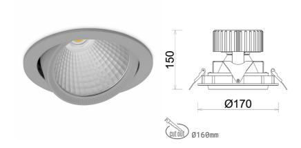
COB Light colour 2700 [K] | CRI Led chip flux 3233 [lm] Luminous flux 2586 [lm] System power 23 [W] Luminaire Efficiency 112 [lm/W] Beam angle 45° Controller ON/OFF MacAdam 3 SDCM
