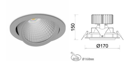
COB 3000 [K] CRI97 Light colour CRI Led chip flux 2601 [lm] Luminous flux 2080 [lm] System power 23 [W] Luminaire Efficiency 90 [lm/W] Beam angle 60° Controller ON/OFF
