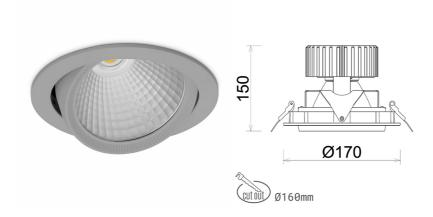
COB 3000 [K] CRI97 Light colour CRI Led chip flux 1575 [lm] Luminous flux 1260 [lm] System power 14 [W] Luminaire Efficiency 90 [lm/W] Beam angle 45° Controller ON/OFF MacAdam 3 SDCM
