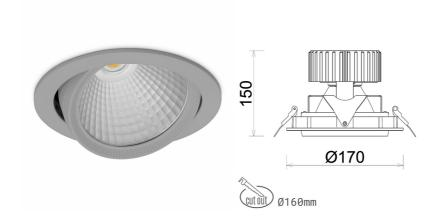
COB 3000 [K] CRI97 Light colour CRI Led chip flux 3735 [lm] Luminous flux 2988 [lm] System power 35 [W] Luminaire Efficiency 85 [lm/W] Beam angle 15° Controller ON/OFF MacAdam 3 SDCM
