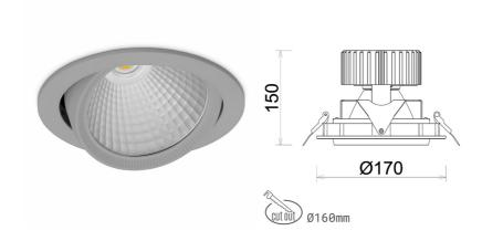
COB 3000 [K] CRI97 Light colour CRI Led chip flux 2402 [lm] Luminous flux 1921 [lm] System power 21 [W] Luminaire Efficiency 91 [lm/W] Beam angle 15° Controller ON/OFF
