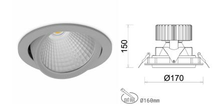
COB 4200 [K] MEAT WHITE Light colour CRI 90 Led chip flux 3040 [lm] Luminous flux 2432 [lm] System power 31 [W] Luminaire Efficiency 78 [lm/W] Beam angle 60° Controller ON/OFF MacAdam 3 SDCM
