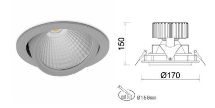
COB 4200 [K] MEAT WHITE Light colour CRI 90 Led chip flux 1023 [lm] Luminous flux 818 [lm] System power 10 [W] Luminaire Efficiency 82 [lm/W] Beam angle 45° Controller ON/OFF
