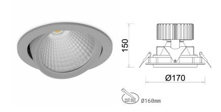
COB 4200 [K] MEAT WHITE Light colour CRI 90 Led chip flux 2519 [lm] Luminous flux 2015 [lm] System power 25 [W] Luminaire Efficiency 81 [lm/W] Beam angle 30° Controller ON/OFF MacAdam 3 SDCM
