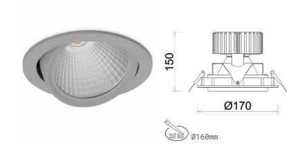
COB 4200 [K] MEAT WHITE Light colour CRI 90 Led chip flux 3539 [lm] Luminous flux 2831 [lm] System power 37 [W] Luminaire Efficiency 77 [Im/W] Beam angle 15° Controller
