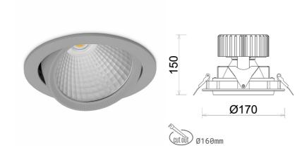
COB 4000 [K] HI EFFICIENT Light colour CRI 90 Led chip flux 2260 [lm] Luminous flux 1808 [lm] System power 14 [W] Luminaire Efficiency 129 [lm/W] Beam angle 45° Controller ON/OFF MacAdam 3 SDCM
