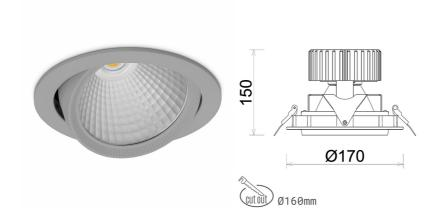
COB 4000 [K] HI EFFICIENT Light colour CRI 90 Led chip flux 5532 [lm] Luminous flux 4425 [lm] System power 34 [W] Luminaire Efficiency 130 [lm/W] Beam angle 30° Controller ON/OFF MacAdam 3 SDCM
