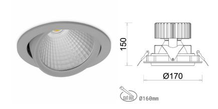
COB 3500 [K] HI EFFICIENT Light colour CRI 90 Led chip flux 5518 [lm] Luminous flux 4414 [lm] System power 36 [W] Luminaire Efficiency 123 [lm/W] Beam angle 45° Controller ON/OFF MacAdam 3 SDCM
