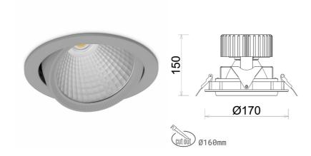
COB 3500 [K] HI EFFICIENT Light colour CRI 90 Led chip flux 4723 [lm] Luminous flux 3778 [lm] System power 31 [W] Luminaire Efficiency 122 [lm/W] Beam angle 30° Controller ON/OFF MacAdam 3 SDCM
