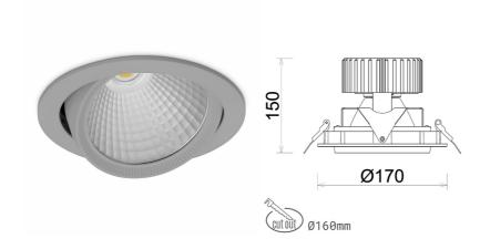
COB 3000 [K] HI EFFICIENT Light colour CRI 90 Led chip flux 5523 [lm] Luminous flux 4418 [lm] System power 34 [W] Luminaire Efficiency 130 [lm/W] Beam angle 60° Controller ON/OFF MacAdam 3 SDCM
