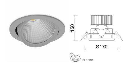
COB 3000 [K] HI EFFICIENT Light colour CRI 90 Led chip flux 4956 [lm] Luminous flux 3964 [lm] System power 31 [W] Luminaire Efficiency 128 [lm/W] Beam angle 60° Controller ON/OFF MacAdam 3 SDCM
