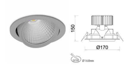
COB 3000 [K] HI EFFICIENT Light colour CRI 90 Led chip flux 1623 [lm] Luminous flux 1298 [lm] System power 10 [W] Luminaire Efficiency 130 [lm/W] Beam angle 60° Controller ON/OFF MacAdam 3 SDCM
