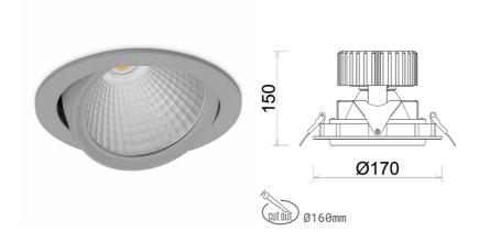
COB 3000 [K] HI EFFICIENT Light colour CRI 90 Led chip flux 3184 [lm] Luminous flux 2547 [lm] System power 19 [W] Luminaire Efficiency 134 [lm/W] Beam angle 45° Controller ON/OFF MacAdam 3 SDCM
