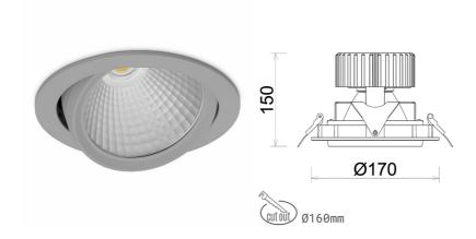
COB 3000 [K] HI EFFICIENT Light colour CRI 90 Led chip flux 5523 [lm] Luminous flux 4418 [lm] System power 34 [W] Luminaire Efficiency 130 [lm/W] Beam angle 30° Controller ON/OFF MacAdam 3 SDCM
