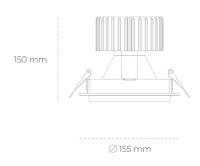
COB Light colour 5000 [K] | CRI Led chip flux 2027 [lm] Luminous flux 1621 [lm] System power 14 [W] Luminaire Efficiency 116 [lm/W] Beam angle 15° Controller ON/OFF MacAdam 3 SDCM
