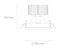
COB 3000 [K] HI EFFICIENT Light colour CRI 90 Led chip flux 2256 [lm] Luminous flux 1804 [lm] System power 14 [W] Luminaire Efficiency 129 [lm/W] Beam angle 60° Controller ON/OFF
