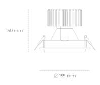
COB 4200 [K] MEAT WHITE Light colour CRI 90 Led chip flux 3040 [lm] Luminous flux 2432 [lm] System power 31 [W] Luminaire Efficiency 78 [lm/W] Beam angle 15° Controller ON/OFF
