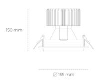
COB 4000 [K] HI EFFICIENT Light colour CRI 90 Led chip flux 5811 [lm] Luminous flux 4648 [lm] System power 36 [W] Luminaire Efficiency 129 [lm/W] Beam angle 60° Controller ON/OFF MacAdam 3 SDCM
