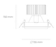
COB Light colour 2700 [K] | CRI Led chip flux 5119 [lm] Luminous flux 4095 [lm] System power 37 [W] Luminaire Efficiency 111 [lm/W] Beam angle 45° Controller ON/OFF MacAdam 3 SDCM
