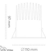
COB 2500 [K] BREAD Light colour CRI Led chip flux 1674 [lm] Luminous flux 1506 [lm] System power 14 [W] Luminaire Efficiency 108 [lm/W] Beam angle 15° Controller ON/OFF MacAdam 3 SDCM
