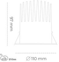
LED downlight for drop ceiling istallation. Aluminium housing. Plastic cover included. Available in white, black and grey. Any RAL palette colour available on enquiry. Reflector beam available: 15°, 23°, 38° and 60°. Maximum power is 27W.
