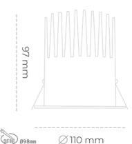
COB Light colour 5000 [K] | CRI Led chip flux 4053 [lm] Luminous flux 3647 [lm] System power 27 [W] Luminaire Efficiency 135 [lm/W] Beam angle 45° Controller ON/OFF MacAdam 3 SDCM
