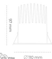
COB 4200 [K] MEAT WHITE Light colour CRI 90 Led chip flux 1976 [lm] Luminous flux 1778 [lm] System power 19 [W] Luminaire Efficiency 94 [lm/W] Beam angle 45° Controller ON/OFF MacAdam 3 SDCM
