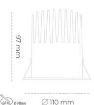
COB 4200 [K] MEAT WHITE Light colour CRI 90 Led chip flux 1976 [lm] Luminous flux 1778 [lm] System power 19 [W] Luminaire Efficiency 94 [lm/W] Beam angle 15° Controller ON/OFF MacAdam 3 SDCM
