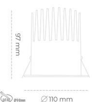
COB 3000 [K] HI EFFICIENT Light colour CRI 90 Led chip flux 3184 [lm] Luminous flux 2865 [lm] System power 19 [W] Luminaire Efficiency 151 [lm/W] Beam angle 45° Controller ON/OFF MacAdam 3 SDCM
