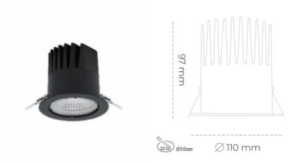
LED Light colour 2000 [K] MEAT PINK CRI 80 Led chip flux 1741 [lm] 1566 [lm] Luminous flux System power 19 [W] Luminaire Efficiency 82 [lm/W] Beam angle 60° Controller ON/OFF
