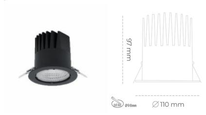
LED 4000 [K] PREMIUM WHITE Light colour CRI 90 Led chip flux 1887 [lm] Luminous flux 1698 [lm] System power 14 [W] Luminaire Efficiency 121 [lm/W] Beam angle 45° Controller ON/OFF MacAdam 3 SDCM
