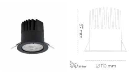
LED 4000 [K] PREMIUM WHITE Light colour CRI 90 Led chip flux 3398 [lm] Luminous flux 3058 [lm] System power 25 [W] Luminaire Efficiency 122 [lm/W] Beam angle 15° Controller ON/OFF MacAdam 3 SDCM
