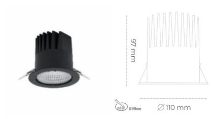
LED 3000 [K] PREMIUM Light colour COLOR CRI 90 Led chip flux 2776 [lm] Luminous flux 2498 [lm] System power 25 [W] Luminaire Efficiency 100 [lm/W] Beam angle 23° Controller ON/OFF MacAdam
