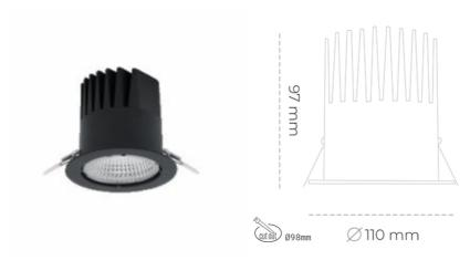
LED 3000 [K] PREMIUM Light colour COLOR CRI 90 Led chip flux 2396 [lm] Luminous flux 2156 [lm] System power 21 [W] Luminaire Efficiency 103 [lm/W] Beam angle 23° Controller ON/OFF MacAdam 3 SDCM
