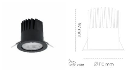
LED 3000 [K] PREMIUM Light colour COLOR CRI 90 Led chip flux 2776 [lm] Luminous flux 2498 [lm] System power 25 [W] Luminaire Efficiency 100 [lm/W] Beam angle 15° Controller ON/OFF MacAdam 3 SDCM
