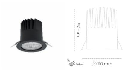
LED 3000 [K] PREMIUM Light colour COLOR CRI 90 Led chip flux 1145 [lm] Luminous flux 1030 [lm] System power 11 [W] Luminaire Efficiency 94 [lm/W] Beam angle 15° Controller ON/OFF MacAdam 3 SDCM
