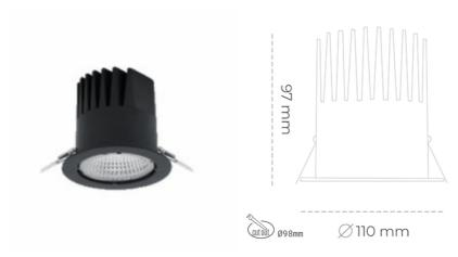
LED 3500 [K] PREMIUM WHITE Light colour CRI 90 Led chip flux 4038 [lm] Luminous flux 3634 [lm] System power 27 [W] Luminaire Efficiency 135 [lm/W] Beam angle 60° Controller ON/OFF MacAdam 3 SDCM
