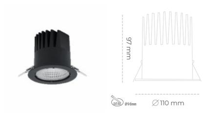
LED 3500 [K] PREMIUM WHITE Light colour CRI 90 Led chip flux 3245 [lm] Luminous flux 2920 [lm] System power 21 [W] Luminaire Efficiency 139 [lm/W] Beam angle 23° Controller ON/OFF MacAdam 3 SDCM
