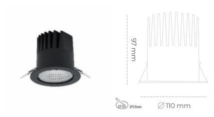
LED 3500 [K] PREMIUM WHITE Light colour CRI 90 Led chip flux 2973 [lm] Luminous flux 2675 [lm] System power 20 [W] Luminaire Efficiency 134 [lm/W] Beam angle 23° Controller ON/OFF MacAdam 3 SDCM
