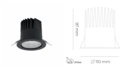
LED 3500 [K] PREMIUM WHITE Light colour CRI 90 Led chip flux 3245 [lm] Luminous flux 2920 [lm] System power 21 [W] Luminaire Efficiency 139 [lm/W] Beam angle 15° Controller ON/OFF MacAdam 3 SDCM
