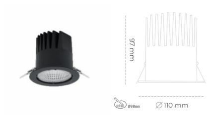
LED 3000 [K] PREMIUM WHITE Light colour CRI 90 Led chip flux 2064 [lm] Luminous flux 1857 [lm] System power 14 [W] Luminaire Efficiency 133 [lm/W] Beam angle 45° Controller ON/OFF MacAdam 3 SDCM
