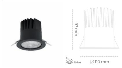
LED 3000 [K] PREMIUM WHITE Light colour CRI 90 Led chip flux 3143 [lm] Luminous flux 2828 [lm] System power 21 [W] Luminaire Efficiency 135 [lm/W] Beam angle 38° Controller ON/OFF MacAdam 3 SDCM
