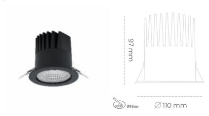
LED 3000 [K] PREMIUM WHITE Light colour CRI 90 Led chip flux 2064 [lm] Luminous flux 1857 [lm] System power 14 [W] Luminaire Efficiency 133 [lm/W] Beam angle 15° Controller ON/OFF MacAdam 3 SDCM
