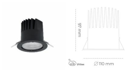
LED COB 4000 [K] HI EFFICIENT Light colour CRI 90 Led chip flux 3492 [lm] Luminous flux 3142 [lm] System power 21 [W] Luminaire Efficiency 150 [lm/W] Beam angle 15° Controller ON/OFF MacAdam 3 SDCM
