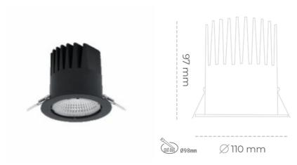
LED COB 4000 [K] HI EFFICIENT Light colour CRI 90 Led chip flux 3189 [lm] Luminous flux 2870 [lm] System power 19 [W] Luminaire Efficiency 151 [lm/W] Beam angle 15° Controller ON/OFF MacAdam 3 SDCM
