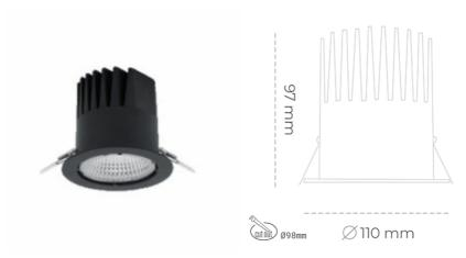
LED COB 3500 [K] HI EFFICIENT Light colour CRI 90 Led chip flux 3054 [lm] Luminous flux 2748 [lm] System power 19 [W] Luminaire Efficiency 145 [lm/W] Beam angle 15° Controller ON/OFF MacAdam 3 SDCM
